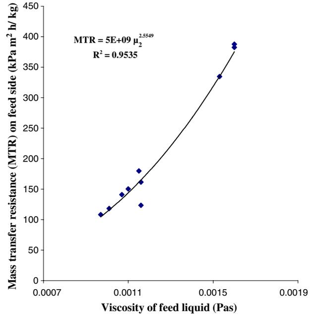
Fig. 11. Impact of feed viscosity on boundary layer resistance ( $R_2$ ).
