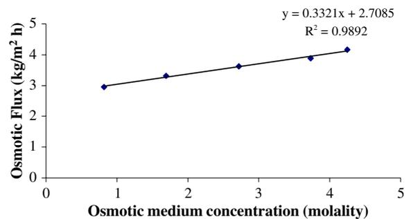
Fig. 6. The effect of osmotic medium concentration on the direct osmotic flux.
