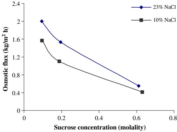
Fig. 8. Impact of feed (sucrose) concentration on osmotic flux.
