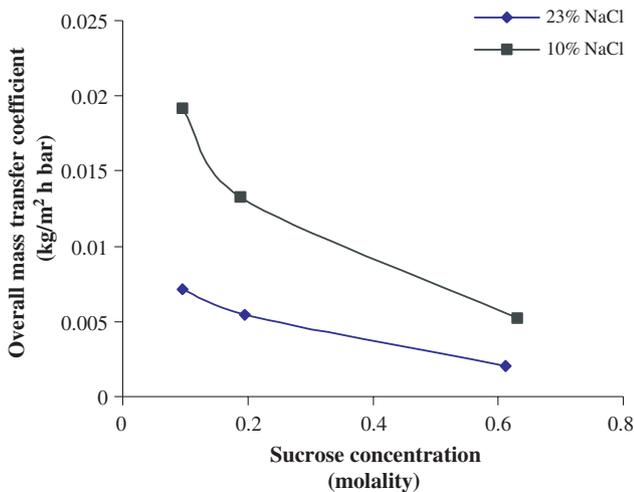
Fig. 10. Impact of feed (sucrose) concentration on overall mass transfer coefficient.
