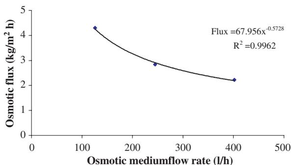
Fig. 13. Impact of osmotic medium flow rate on osmotic flux.
