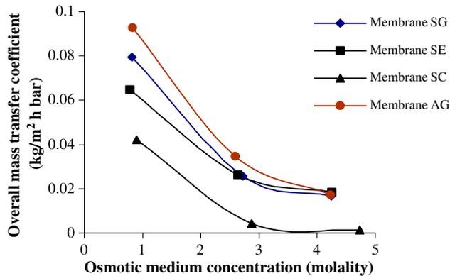
Fig. 5. Impact of membrane type (characteristics) and osmotic medium concentration on overall mass transfer coefficient ( $U$ ).
