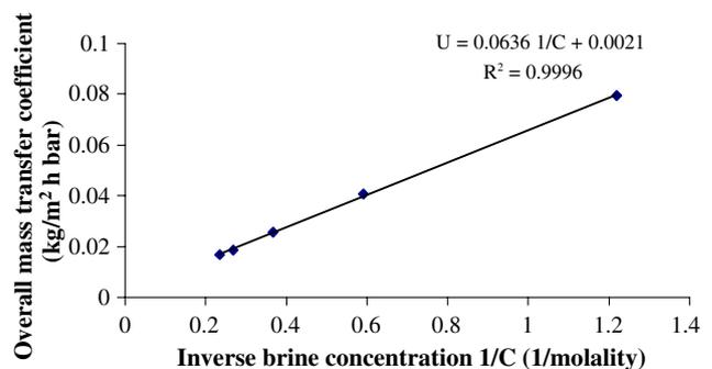
Fig. 7. Impact of osmotic medium concentration on overall mass transfer coefficient.
