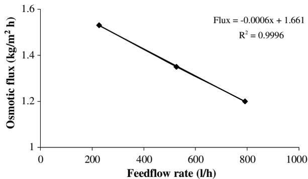
Fig. 12. Impact of osmotic feed flow rate on osmotic flux.
