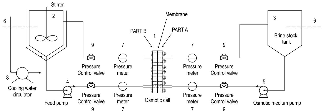
Fig. 1. Schematic diagram of experimental set up for direct osmosis.
