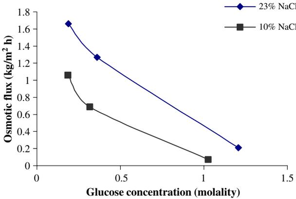
Fig. 9. Impact of feed (glucose) concentration on osmotic flux.
